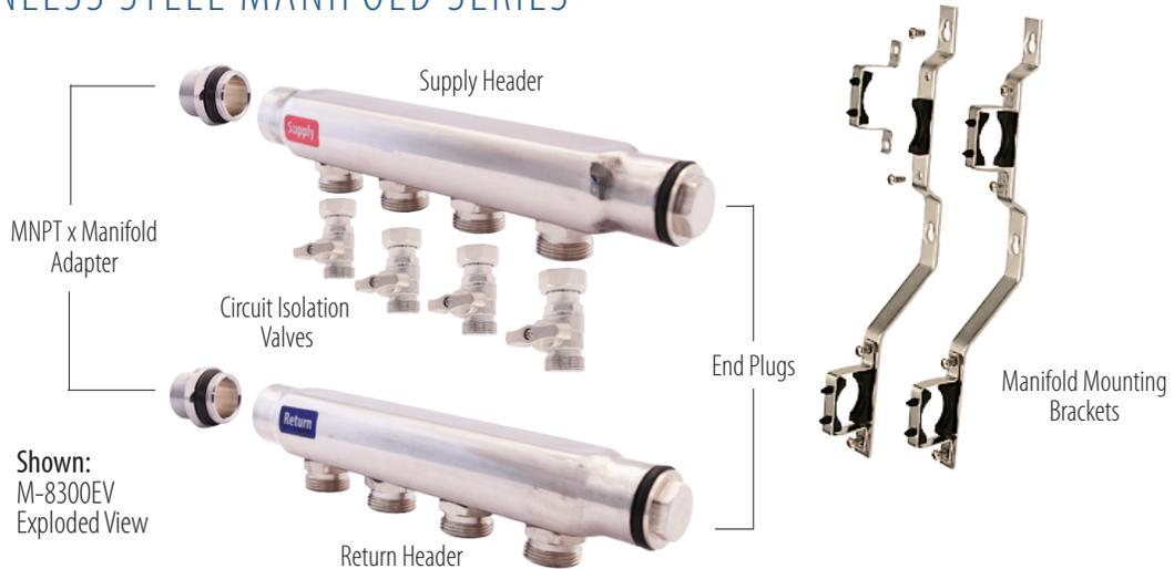
The M-8300EV Stainless™ Manifolds are designed for use in hydronic heating and cooling applications that do not require individual circuit flow control and are available in various sizes up to 12 circuits. Projects using these manifolds must be self balancing or have other means to balance the individual loops.
